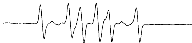
Figure 5. ESR spectrum of the reaction mixture of (\text{OC})_5\text{CrMn}(\text{CO})_5^- \text{PPN}^+ with \text{CH}_2\text{CHCH}_2\text{Br} in THF in the presence of DMPO at ambient temperature.
