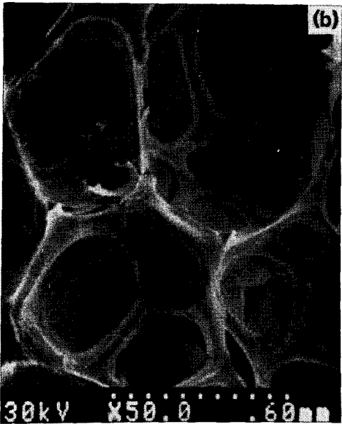
Fig. 4. S. E. M. photographs of carbon coated poly-urethane (27ppi) foam. (a) 15 : 1 (b) 5 : 1
