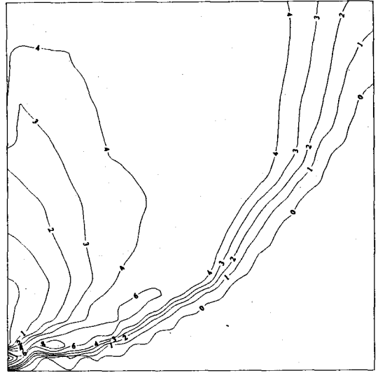
Fig. 14. Plan view of excess temperature field. (Crossflow: 2 m/sec 2.5 m below the free surface)
