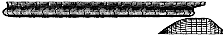
Figure 2.a Surface panel representation of the Sydney Express ship model with the flow liners(side view, N_S=20, M_S=17, N_F=20, M_F=10, N_W=20, M_W=10 ).
