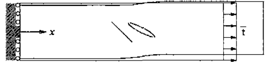
Fig. 6 Initial and deformed shape of a centered 45° slant crack in a rectangular plate subjected to tension ( h/b=3.5 , a/b=0.5 )
