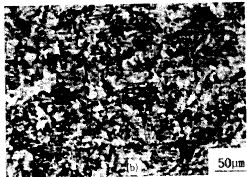
Fig. 7 Grain size (a) and microstructure (b) of SUP 9A(20% reduction ratio)
