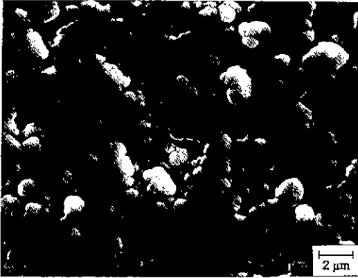
Fig. 4. Scanning electron micrograph of the as-deposited WO 3 thin film (×5000).
