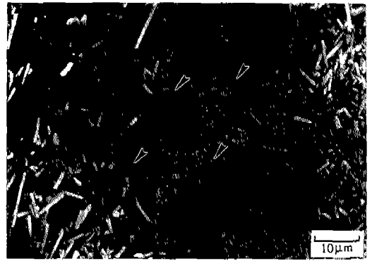
Fig. 5. SEM micrograph of the 2124 Al-SiC w composite, showing coarse Mn-containing intermetallic particles. 13)
