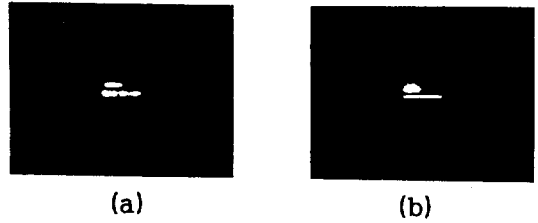
그림 4. Reconstructed images from the hologram recorded by scanned-object holography. Since the object was composed of two lines placed at different positions, different images are obtained according to the position of an observation plane, and both a sharp and a defocused image of two lines are shown from each photograph. They are (a) the sharp image of the short line placed at the near position from the recording material and (b) that of the long line at the distant position.
