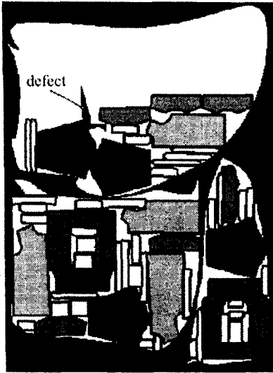
Fig. 16 Nesting of 56 patterns on three irregular sheets one of which has an interior defect (wr =26.3%, cpu=1198 sec on 16 Mips EWS)
