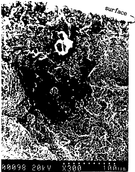
Fig. 8(a) SEM fractograph showing a crack initiation site
