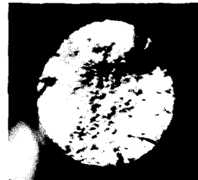
Fig. 3 Macrofractograph in SM55C specimen (smooth, \sigma_{max}=482 MPa, N_f=4.4 \times 10^4 )
