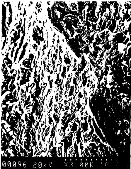
(b) Ductile fracture(smooth, \sigma_{\max}=424 MPa, N_f=7.44 \times 10^4 )
