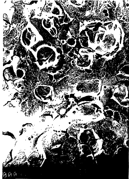
Fig. 8(d) Cluster of inclusions contributing to brittle fracture
