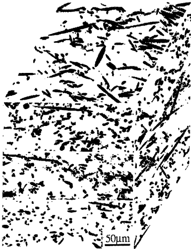
Fig. 2 Microstructure of Al 2 O 3 /Al composites made by squeeze casting
