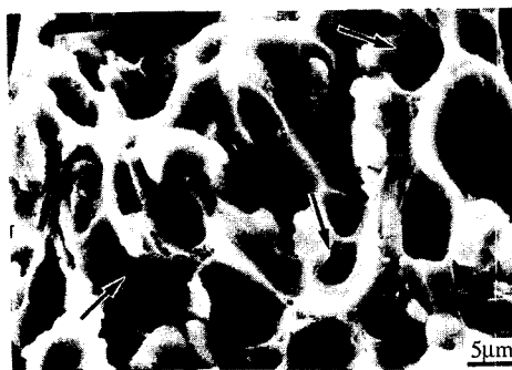
Fig. 11 SEM photographs of fractured surface for Al 2 O 3 /Al composites
