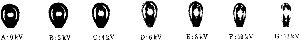
Fig. 5(c) Deformed shapes of a bubble in Type 3
