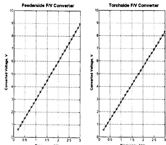
Fig. 5 Calibration Chart of Wire Feedrate Measuring System
