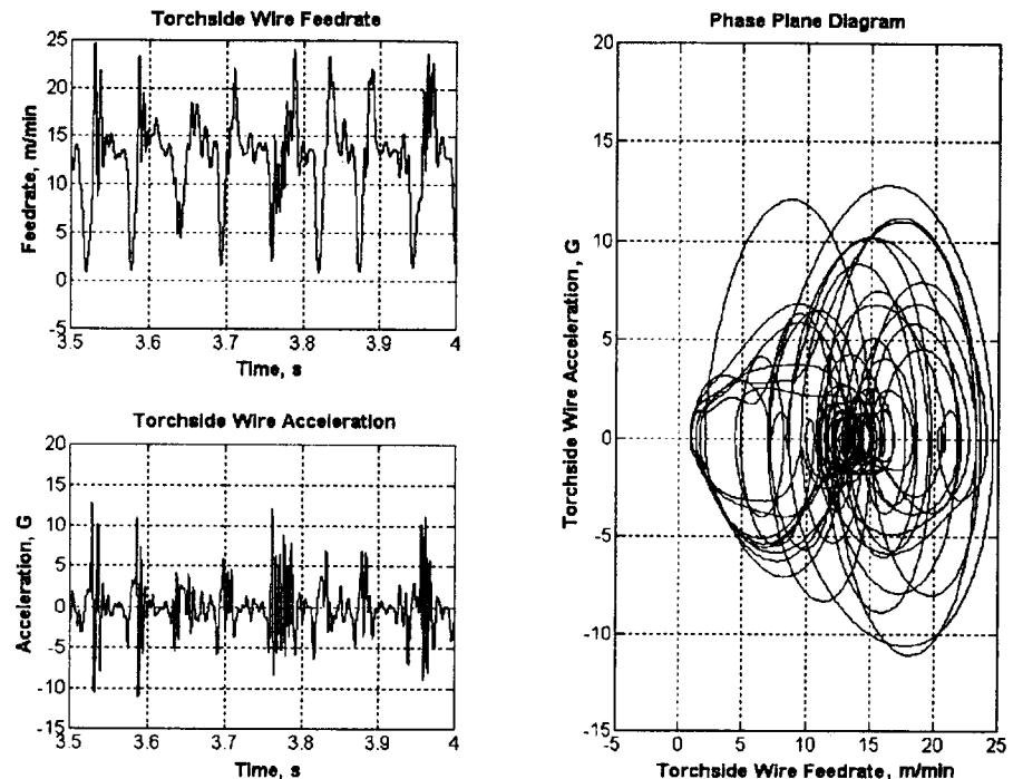
Fig. 10(c) Phase Plane Diagram of Torch-side Wire Feed Rate( $v_w$ ) ( $\text{CO}_2$ , Current=350A, Voltage=LowMid Range)
