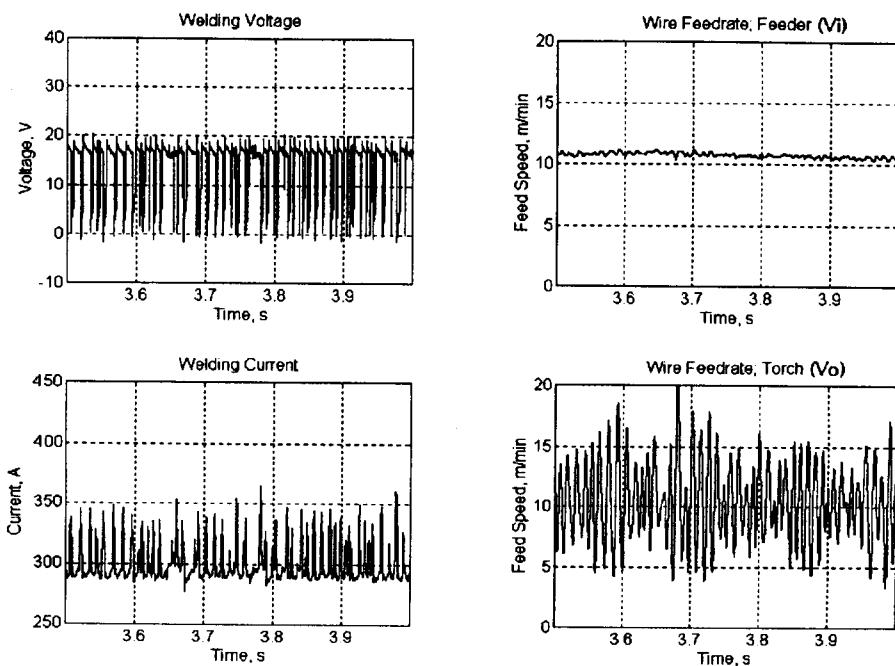
Fig. 6(d) Typical Time Records of Process Parameters in GMA Welding ( $I=300A$ , CO<sub>2</sub> Shield)
