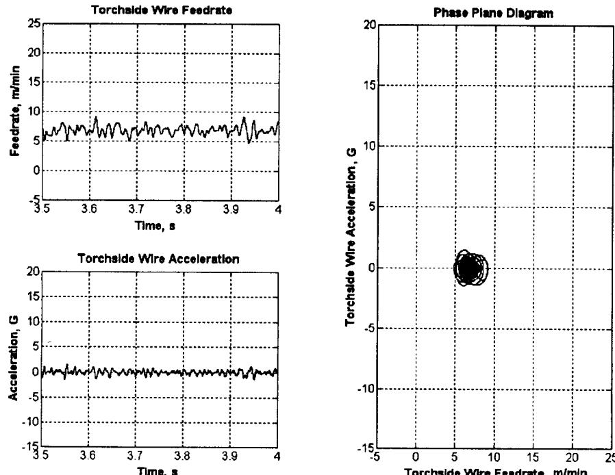
Fig. 10(a) Phase Plane Diagram of Torch-side Wire Feed Rate( $v_o$ ) (CO<sub>2</sub>, Current=250A, Voltage=MidHigh Range)
