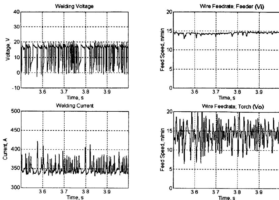
Fig. 6(e) Typical Time Records of Process Parameters in GMA Welding ( $I=350A$ ,  $\text{CO}_2$  Shield)
