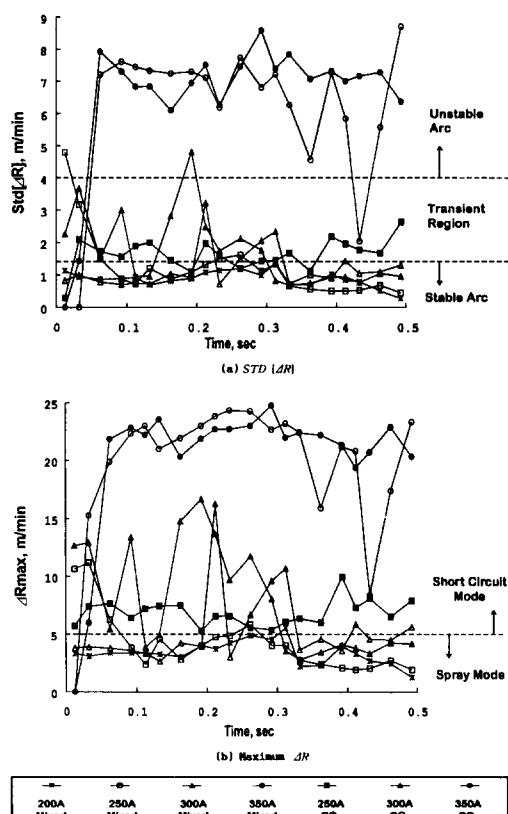
Fig. 8 Std [ $\Delta R$ ] and Maximum  $\Delta R$  for Various Welding Conditions
