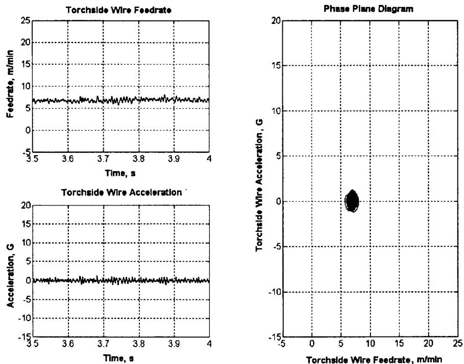
Fig. 10(b) Phase Plane Diagram of Torch-side Wire Feed Rate( $v_w$ ) ( $\text{CO}_2\text{-Ar}$  Mixed, Current=250A, Voltage=MidHigh Range)
