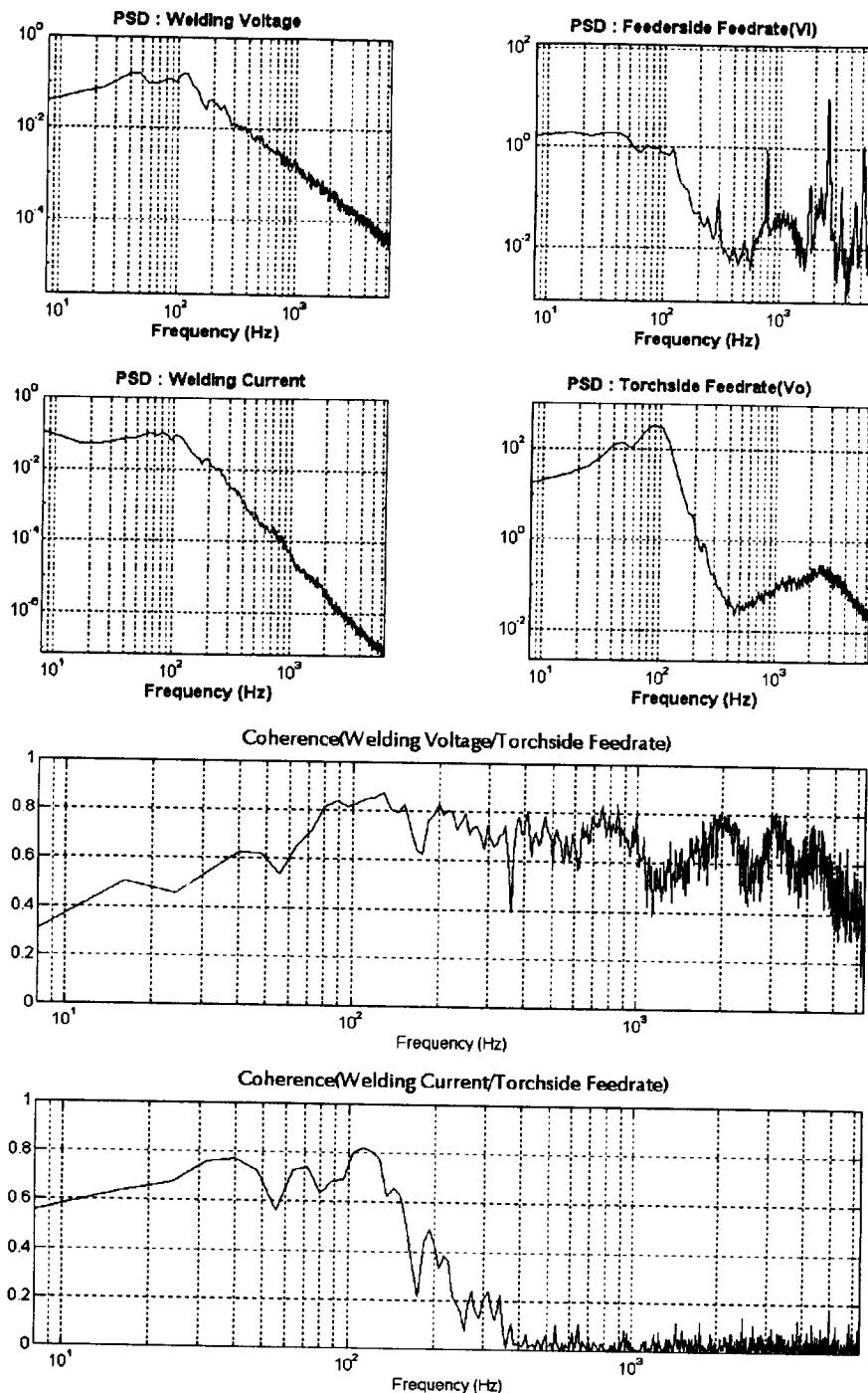
Fig. 9(d) PSD Plots for Various Process Parameters and Coherence between Voltage(Current) and Torch-side Wire Feed rate,  $v_o$  (Welding Current = 350A)
