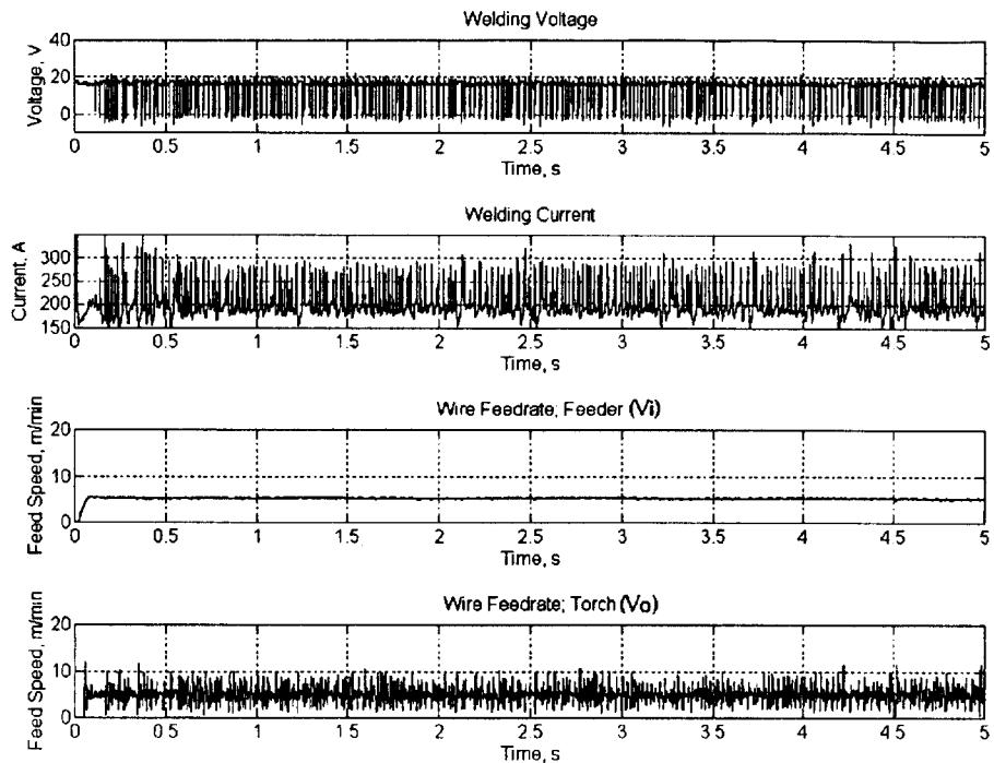
Fig. 6(a) Time Records of Process Parameters in GMA Welding ( $I=200A$ ,  $\text{CO}_2$  Shield)
