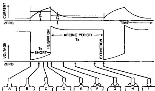
Fig. 1 Short Circuiting Transfer in GMA Welding Processes
