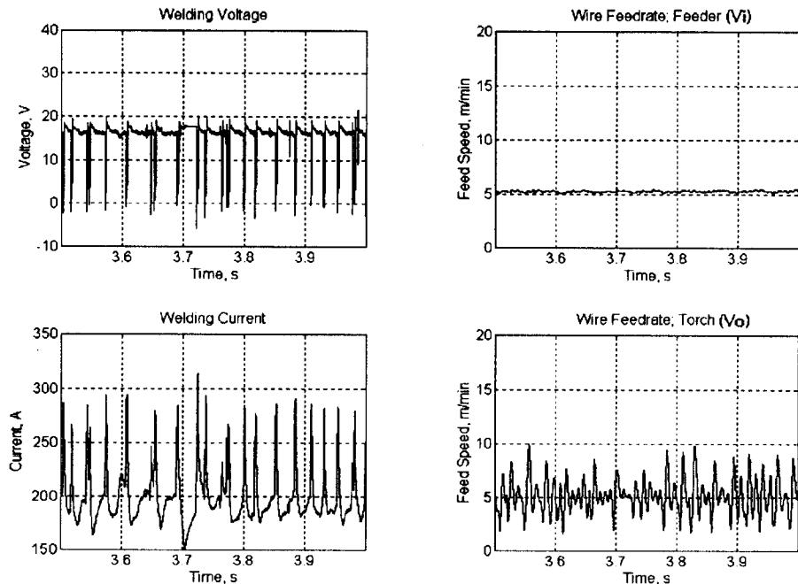
Fig. 6(b) Typical Time Records of Process Parameters in GMA Welding ( $I=200A$ ,  $\text{CO}_2$  Shield)
