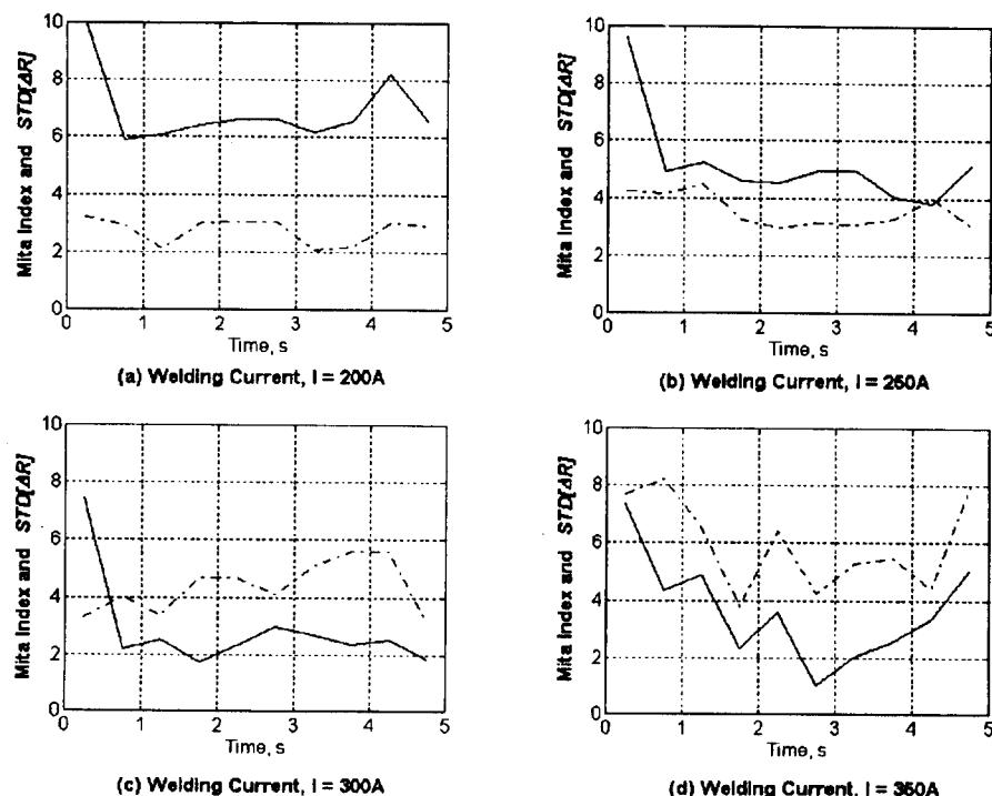
Fig. 7 Mita Index and Wire Feed Speed Fluctuation during GMA Welding( $\text{CO}_2$  Shield)
