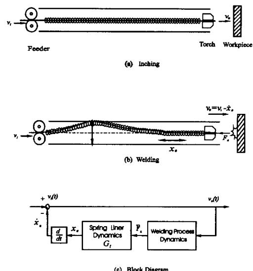
Fig. 3 Schematic Diagram of Spring Liner System
