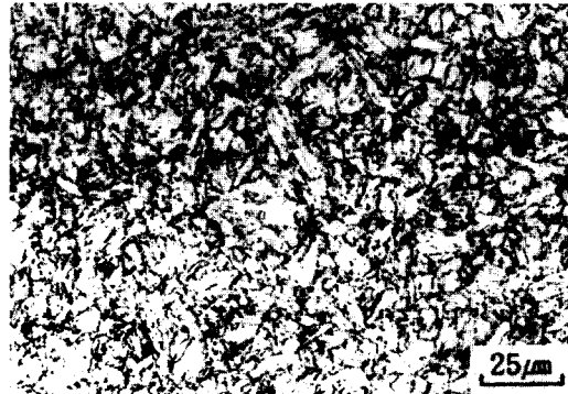
Photo.1 Microstructure of 9% Ni steel
