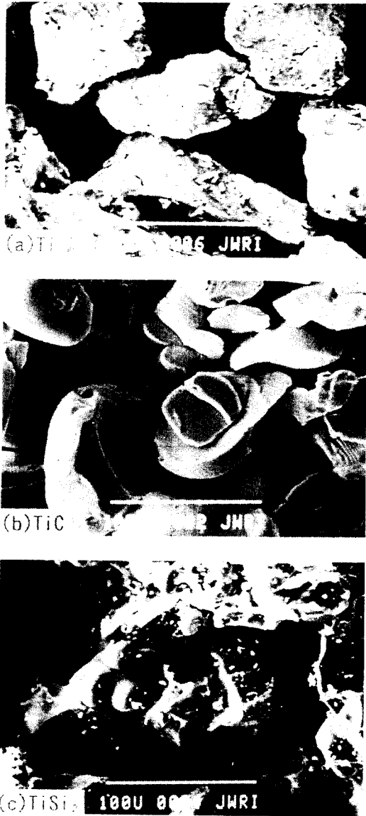
Photo. 1 Shape of powders(SEM)
