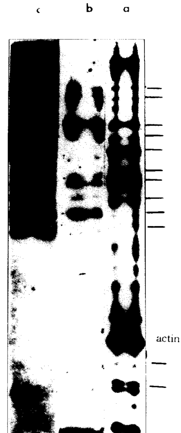
Fig. 8. Immunoblotting of RNA polymerase II subunits separated by sodium dodecylsulfate-polyacrylamide gel electrophoresis. Lane a: RNA polymerase II was visualized with a silver stain after electrophoresis in 6%/8% SDS-PAGE; Lane b: The RNA polymerase II blot was treated with affinity purified IgY, I-labelled protein A, washed, dried, and autoradiographed; Lane c: The identical blot was treated with DEAE-cellulose purified IgY.
