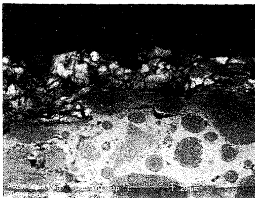
Fig. 50 Back scattered image of cutting surface of Dispersalloy amalgam after 6 months in artificial saliva
