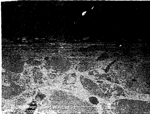
Fig. 48 Back scattered image of cutting surface of Cavex 68 amalgam after 6 months in artificial saliva
