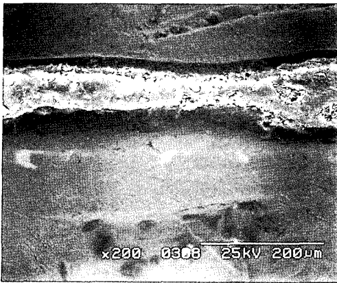
Fig. 7. Scanning electron microscopy at A&B marking points after cemented with All-Bond& composite resin cement.
