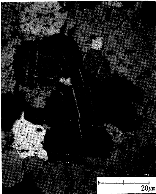
Fig. 10. Ilmenite (il) with veinlets of hematite (hem) in the massive iron ore.
