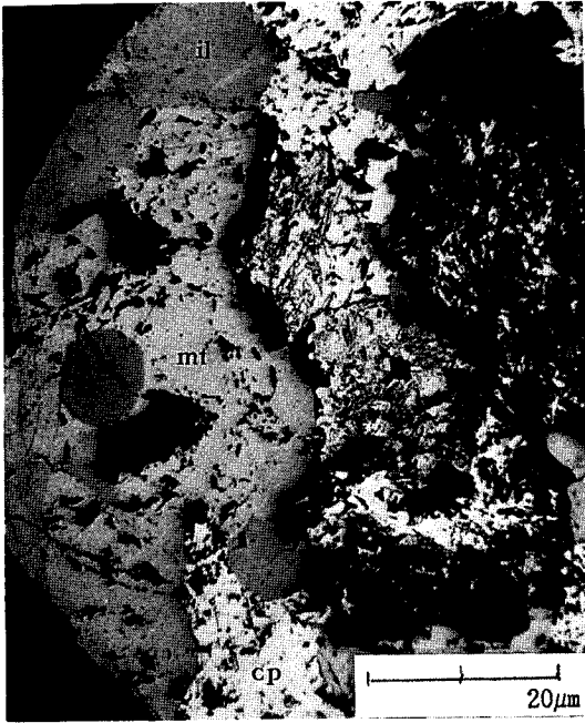
Fig. 9. Coexisted titanomagnetite (mt) and ilmenite minerals, A small amount of chalcopyrite (cp) are associated with iron ore minerals.
