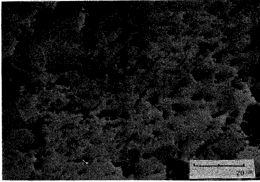
Fig. 9. Titanomagnetite with exsolutions of ilmenite in the titanomagnetite iron ore.
