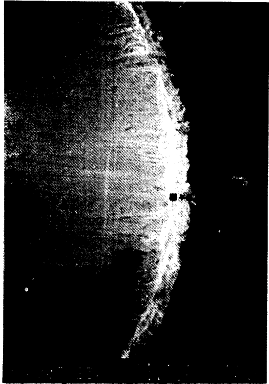
Photo 1. A SEM micrographs of oxidized W/Al alloy interface.
