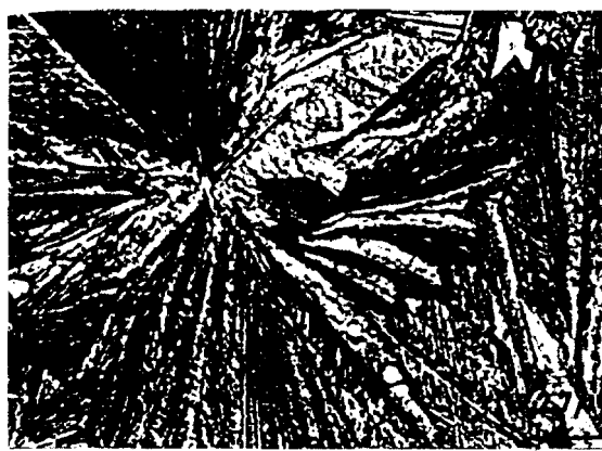
Figure 9. Microstructure of benzidine-catechol eutectic ( E_1 ) \times 100 .
