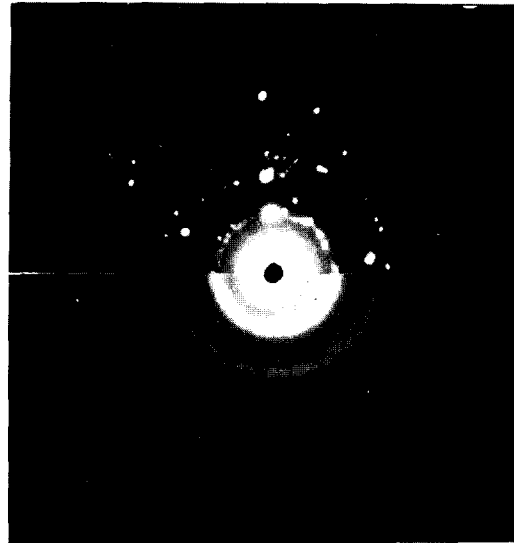
Fig. 3. Electron diffraction patterns obtained from polycrystalline(lower) and amorphous(upper) silicon powder.
