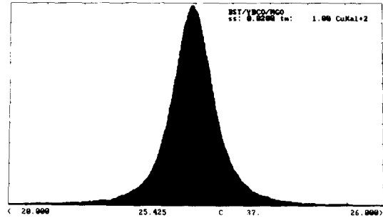
Fig. 2. XRD \omega rocking curve of BST (200) thin film on YBCO/MgO substrate (FWHM : 0.719)
