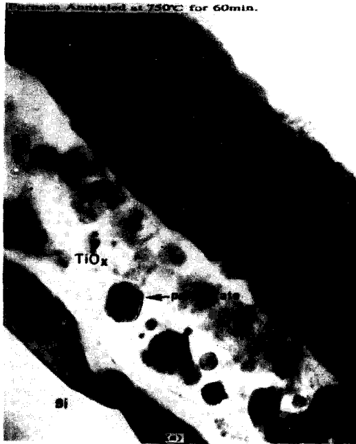
Fig. 8. Cross-sectional view of PZT thin films furnace annealed at 750°C for 60min on Pt(1000Å)/Ti/Si substrate by scanning transmission electron microscopy (STEM)
