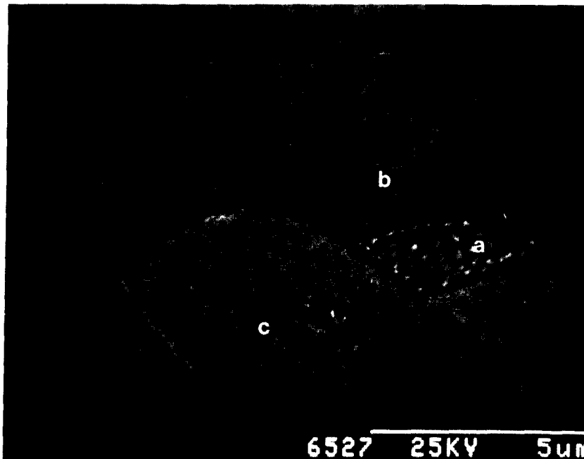
Fig. 3. SEM micrograph of the three different types morphologies of the C49 TiSi 2 , which are (a) randomly spread small islands, (b) connected intermediate size islands, and (c) uniform coverage (two dimensional-like) islands.
