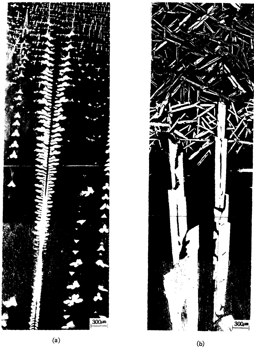
Fig. 9. Sb- and InSb-primary dendrite growing unidirectionally in off-eutectic alloys of 26wt.%In (a), and 34wt.%In (b), ( R=2.7 \times 10^{-3} cm/s).
