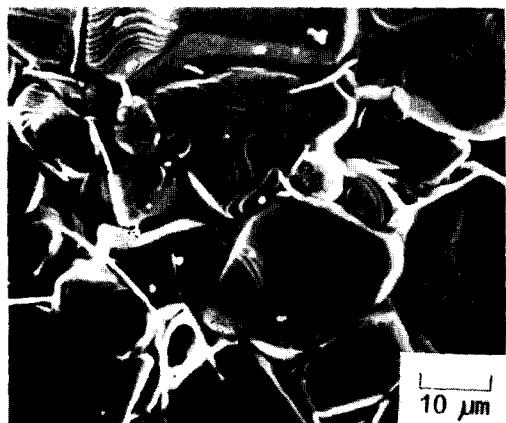
Fig. 6 SEM photographs of fibrous powder and fractured ceramic surfaces of (a) 0.2 \mu\text{m} , (b) 1.2 \mu\text{m} and (c) 2.0 \mu\text{m} BaTiO 3
