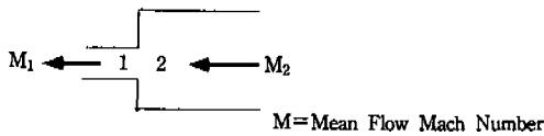
Fig.8 Acoustic model of sudden contraction of a tube in the presence of mean flow.
