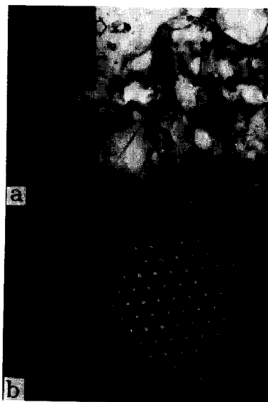
Fig. 10. (a) TEM micrograph showing the \text{Sm}(\text{Fe}, \text{Mo})_7 grains, and (b) is a electron diffraction pattern obtained from (a). The inset in (a) is a microdiffraction pattern obtained from the \text{Fe}_3\text{Mo} particle indicated by an arrow.
