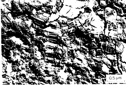
Fig. 1. Electron micrograph of a fractured PTFE surface.
