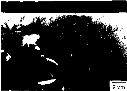
Fig. 11. Cross-sectional image of MgO thin film on Si(100) substrate. The deposition conditions are; substrate temperature: 600°C, pressure: 10 mtorr, RF input power density: 5 W/cm 2 , Ar/O 2 : 50/50.
