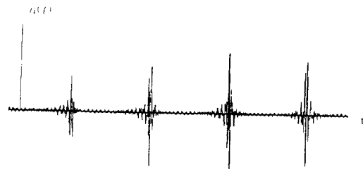
Fig. 2 The Calculated Noise Wave from Thyristor Circuit. (band width=6 KHz, center freq=120 KHz)
