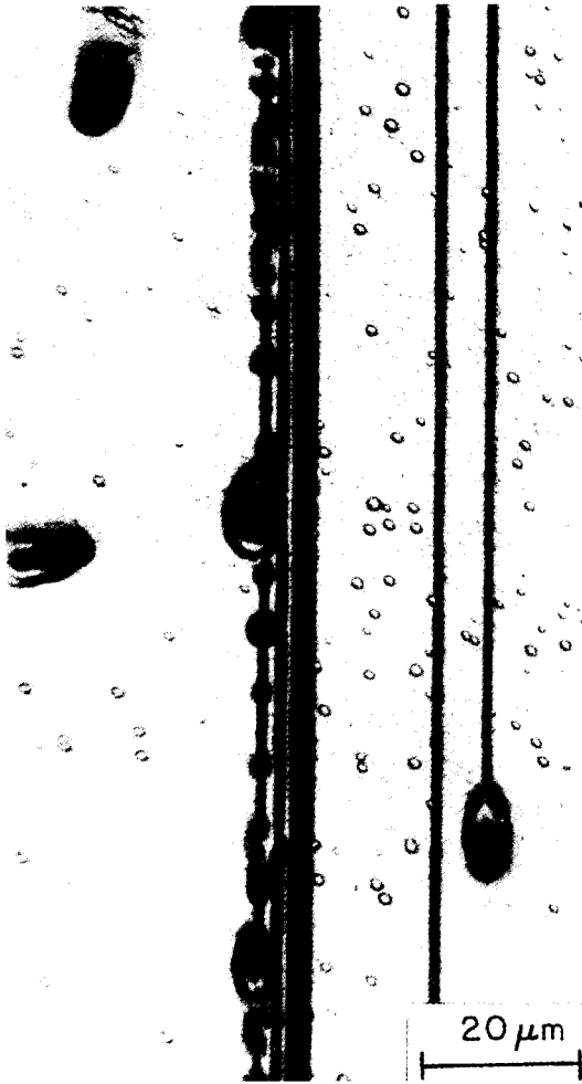
Fig. 10. Optical micrograph of (011) plane showing twin planes, dislocations on the twin plane and portions of two large faulted dislocation loops. Dash solution for 30 min.
