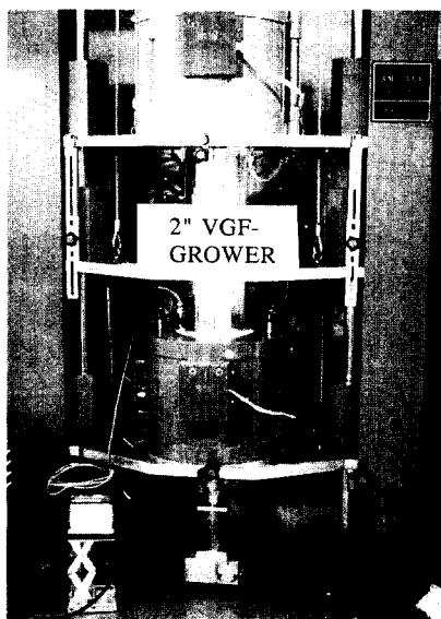
Fig. 1. Photograph of the VGF grower for 2 inch diameter GaAs single crystal.
