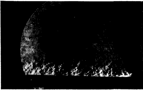
Fig. 6 Schlieren photographs for H=8.5 mm and Re_j=7.24 \times 10^4
