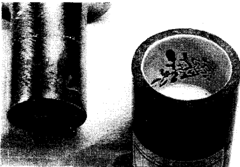
Fig. 13 Photograph of the fracture shape of the circular adherends
