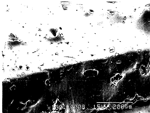
Figure 7 —Surface morphology of EVA matrices containing 20% alginate and 20% of 5-FU: (a) before release, (b) after release experiment for 24 hours.
