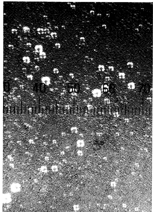
Fig. 3. The polarizing microphotograph of O/W emulsion prepared with long chain alcohol and mixed nonionic surfactants at 25°C. (Nikon OPTIPHOT-POL HFX-II A, ×100)
