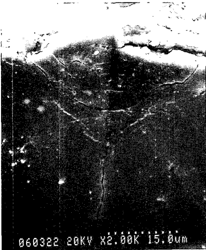
(b) Vickers indentation pattern of the fracture surface ( \times 2000 ).
