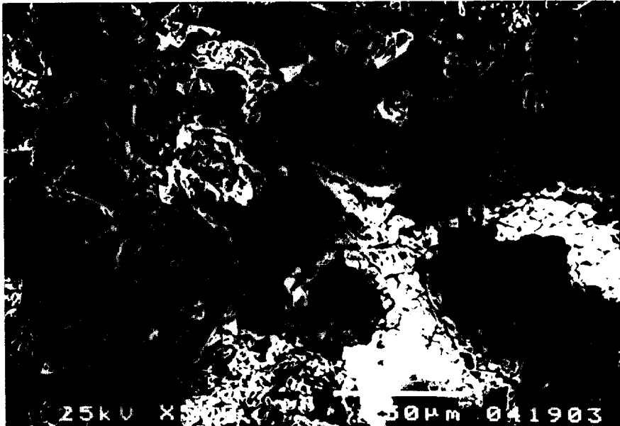
Fig. 7 Scanning electron micrograph of the 200-cycled electrode with 10wt% sealant
