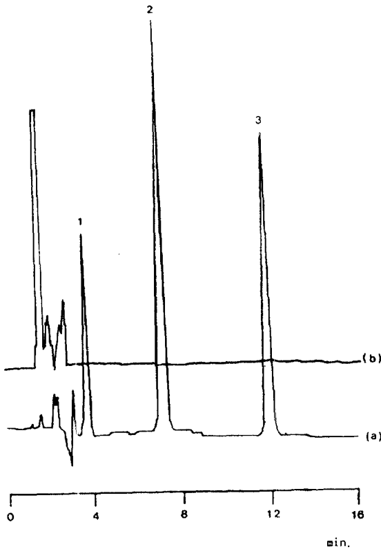
Fig. 2. (a) Typical HPLC Chromatogram of standard solution. : 1. Benomyl 2. Topsin-M 3. Thiram, (b) Typical HPLC Chromatogram of unspiked bean sprouts sample.
