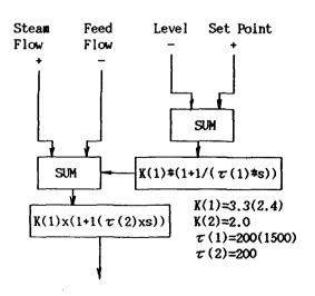
Fig. 1. PI Controllers for Main FW Valve
