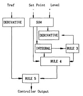
Fig. 8. Fuzzy Logic Controller (Low Power Case)
