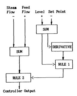
Fig. 3. Fuzzy Logic Controller (High Power Case)
