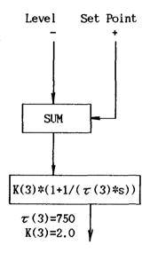
Fig. 2. PI Controller for FW Bypass Valve
