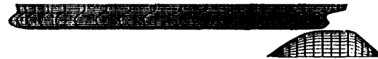
Fig. 2.a Surface panel representation of the Sydney Express ship model with the flow liners (side view, N_S=20, M_S=17, N_F=20, M_F=10, N_W=20, M_W=10 ).
