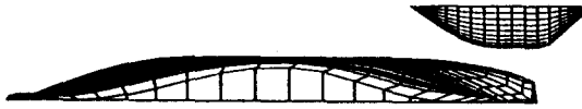
Fig. 2.c Surface panel representation of the Sydney Express ship model with the flow liners (bottom view, N_S=20 , M_S=17 , N_F=20 , M_F=10 , N_W=20 , M_W=10 ).
