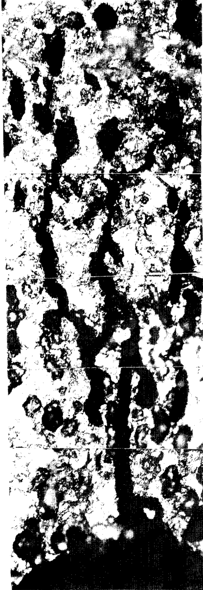
Fig. 6 The shape of crack growth(3.5% NaCl, 182 MPa, 5 \times 10^5 Cycles, Magnification \times 200 )
