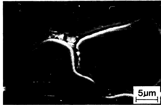
Fig. 5. SEM micrograph of microcracks in tetragonal composition after poling.
