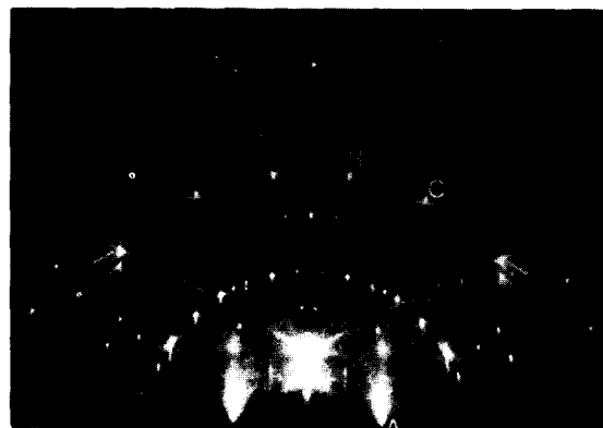
Photo. d. Si(111) 6 \times 1 -Ag structure, azimuth [\bar{1}1\bar{2}] ( \theta=1\text{ML} , T_s=RT ).
