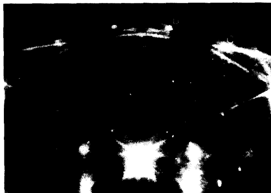
Photo. b. Si(111) \delta 7 \times 7 -Si structure, azimuth [\bar{1}1\bar{2}] .
