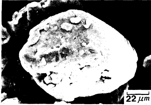
Photo 1. SEM morphologies of the Al-8wt%Fe powders mechanically alloyed for 1300min.
