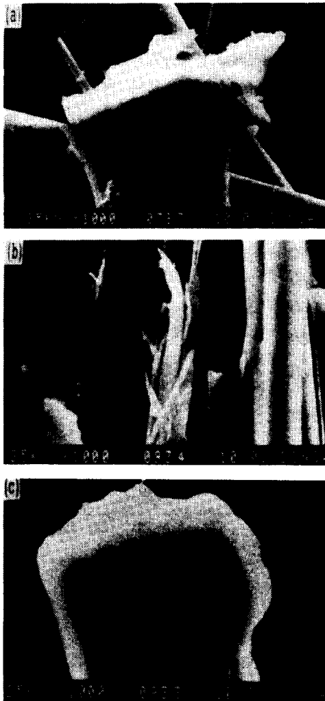
Photo. 1. SEM micrographs of the rupture surface of unknotted netting twines in tensile test. (a) nylon (b) kevlar 29 (c) techmilon
